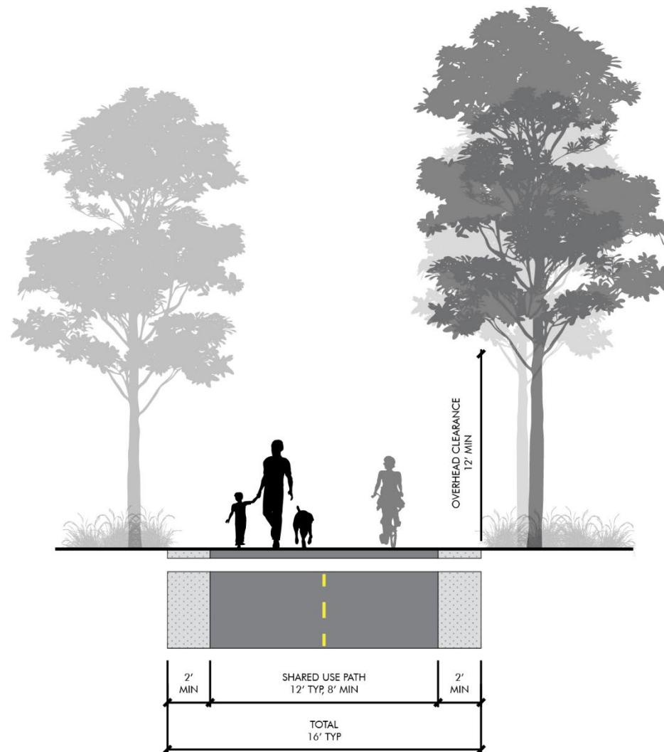
Figure 2-135 Example Cross-Section: FORTAG with No Side Path
